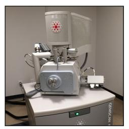
Hazen's new QEMSCAN facility at the Huffman Hazen site (Golden, Colorado) is operational. The system is based on a FEI Quanta 650F scanning electron microscope (SEM), with a large specimen chamber, two Bruker XFlash 6 | 30 high-speed energy dispersive x-ray spectrometers (EDS), and state-of-the-art automated quantitative image analysis and microanalysis software.
