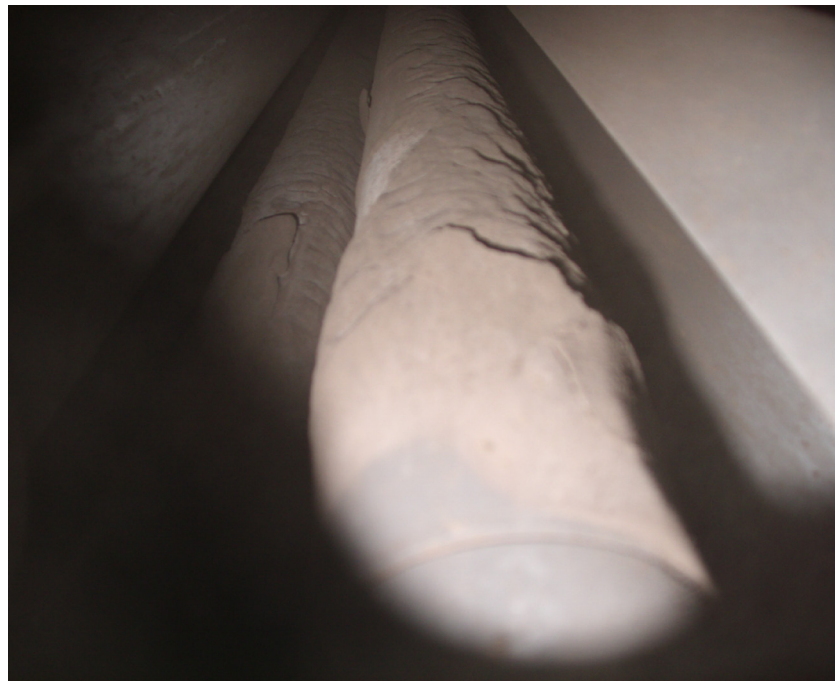
Figure 6. Filter Candles Encrusted with a Mixture of Tar and Solids
